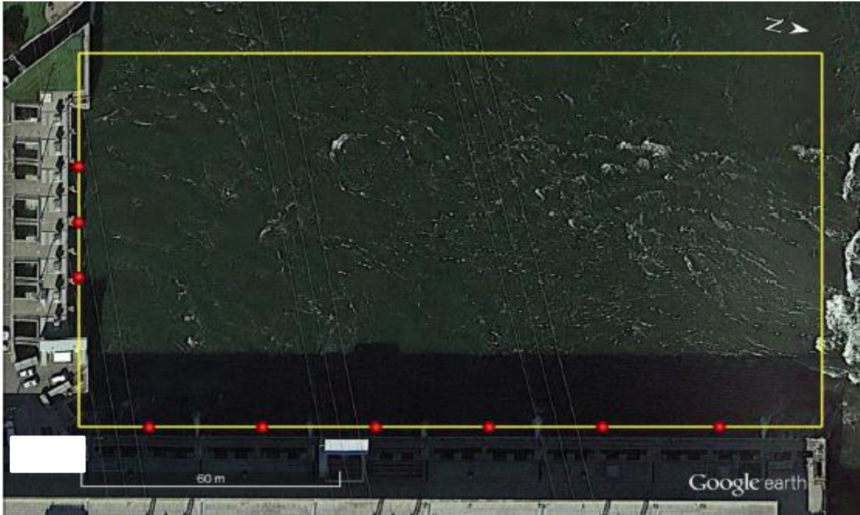
Figure 3.5. Location of an 8 ft x 12 ft (or larger) environmentally controlled equipment trailer to be installed near the tailrace deck of IHR. NOTE: The trailer is not to scale but indicates the approximate location.
