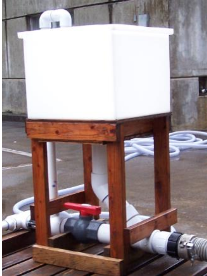
Figure 3.14. Holding tank for fish injection system.
