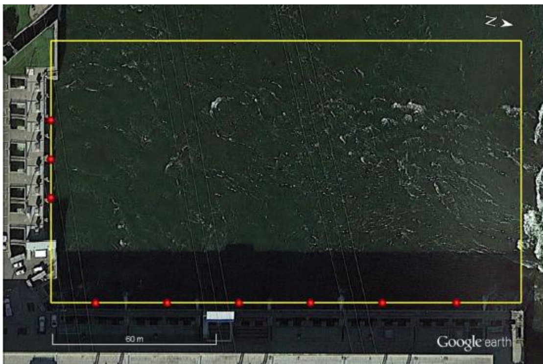
Figure 3.3. Location of the cabled hydrophones in the tailrace of IHR. A deep and shallow hydrophone will be deployed at each location (red dot).
