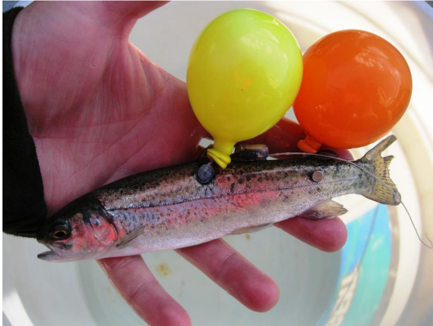
Figure 3.22. Juvenile salmonid equipped with a radio transmitter and two balloon tags.
